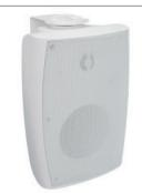
The L-PWP40A is a 40 W cabinet loudspeaker intended for general indoor and outdoor applications. It can recreate original audio effects, and foreground and background music, with precision. There are three types of speaker inputs, and 8 ohm, 70V units are suitable for either high or low voltage audio signal inputs. The cabinet is available in charcoal or white.
