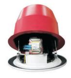
The L-VCM6B/EN is a loudspeaker designed for flush in ceiling mount. It is ideal for even sound distribution. The loudspeaker has a built-in protector to ensure that, in the event of fire, damage to the loudspeaker does not result in failure of the loudspeaker circuit which is connected. System integrity is maintained, ensuring loudspeakers connected in the same circuit in other areas can still be used to inform people of the situation.
